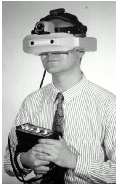
Fig. 2. The Vision Enhancement System developed by Massof et al. allows patients that suffer from macular disease to perceive a high contrast version of the world, with style.
