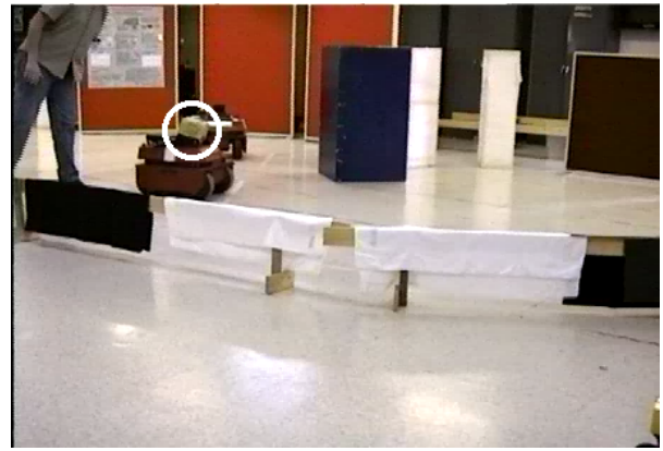
Fig. 5. Placing a box on the cameras triggers an environmental failure
