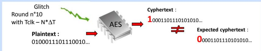
Fig 2. Measurement of path delay for the first bit of the AES.
