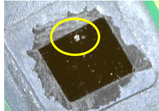
Fig. 4 : Damaged circuit (hole in silicon)
