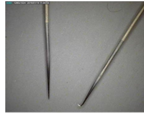
Fig. 5 : Correct and damaged probe tip ends
